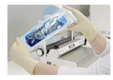
The MELAcontrol Ink test is a reliable test for performing a weekly routine check of the seal seam for leaks in accordance with DIN EN ISO 11607-1 and ASTM F1929-12.
